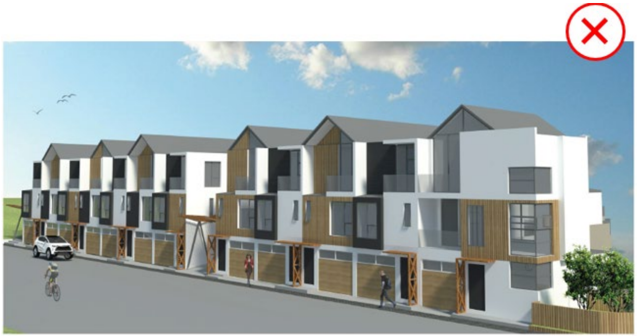
Image 5: Ground level street interface is dominated with garage doors, with no opportunity for landscape treatment or passive surveillance.
