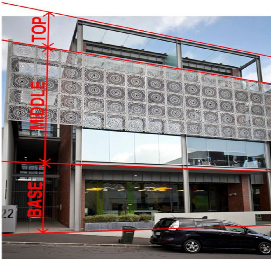
On taller or larger buildings different materials or elements can be utilised to visually break up building height or mass.
