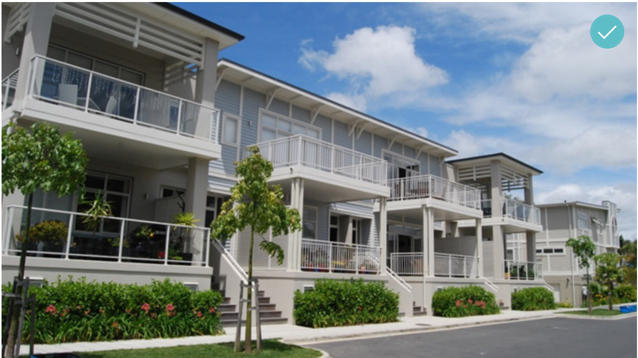
Raising the level of outdoor living areas on the street improves privacy for the occupants while still providing good opportunities for passive surveillance.
