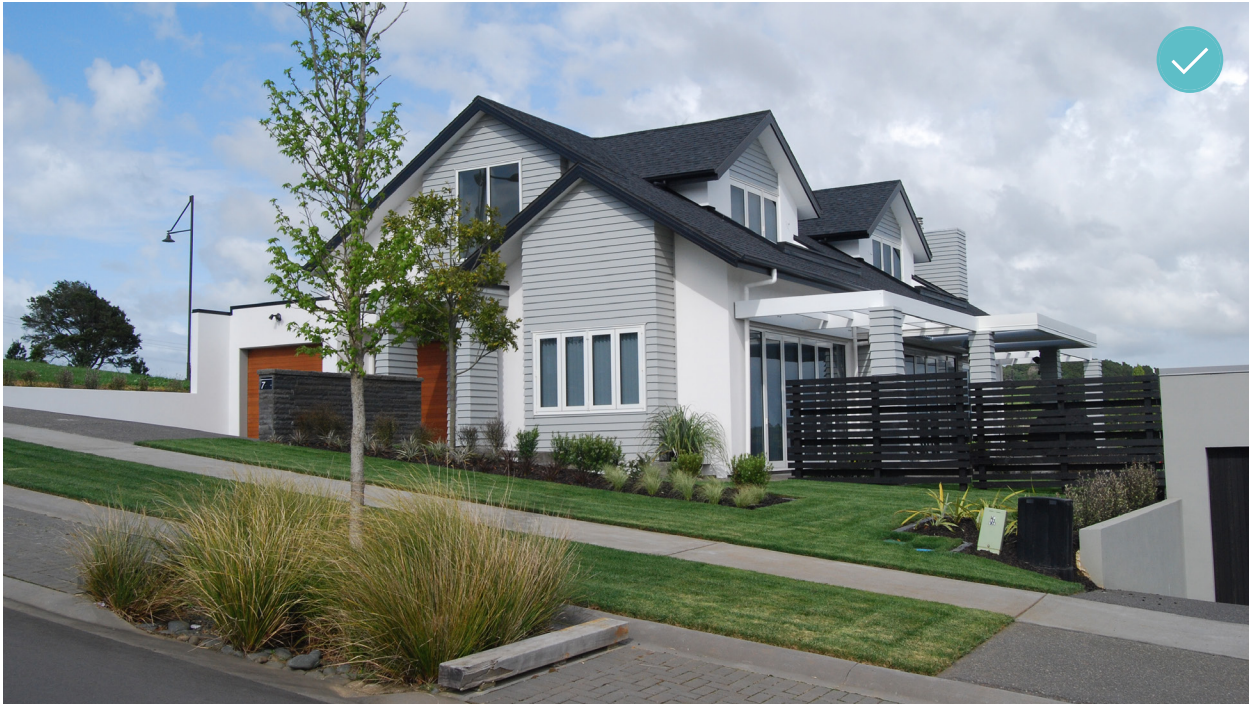
Fencing is avoided in the front yard, with low planting used to define the public/private boundary and fencing set back behind the front façade of the dwelling.
