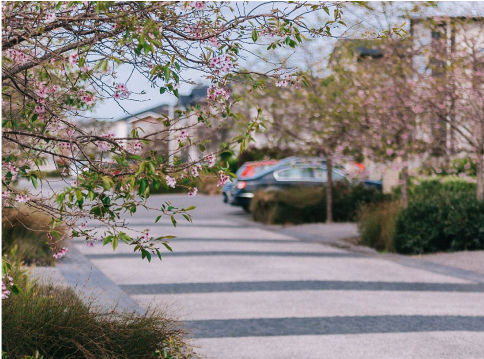
This local street is defined by different surface treatment that encourages slow vehicle speeds. Image credit: Boffa Miskell – Long Bay residential development
