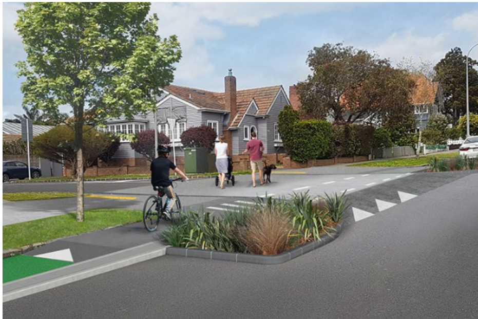
Raised table in different material coupled with the use of planting, signals the entrance to this local road with a slower vehicle environment. Image credit: Artist impression for Boffa Miskell
