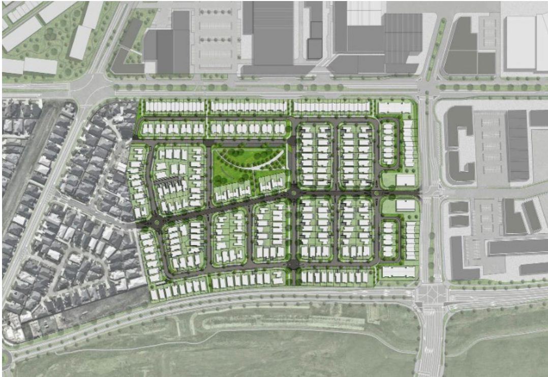
Design the subdivision to connect to existing streets and roads and provide straightforward routes to desired destinations. Image credit: Konstrukt Architects – East Quarter masterplan
