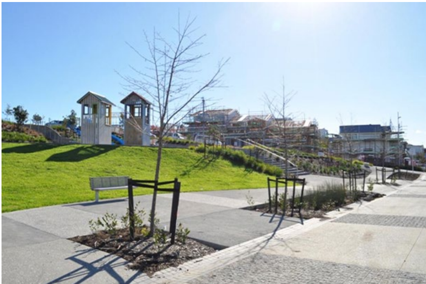
Well-designed development works with existing topography and minimises earth working and the need for retaining structures.
