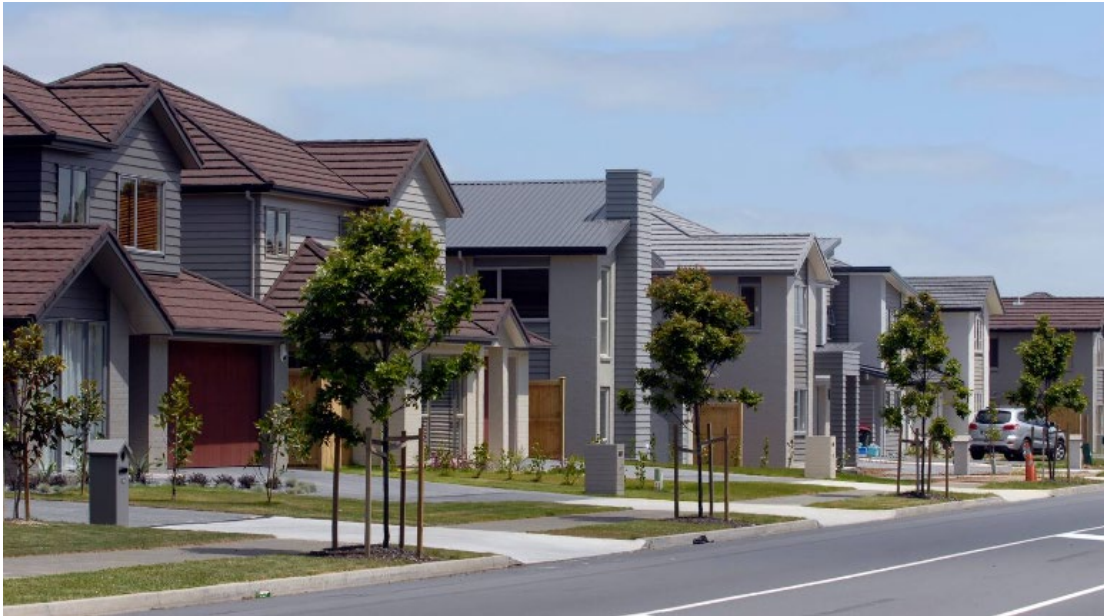
Vehicle crossings that maintain the level of the footpath promote walkable neighbourhoods. Image credit: Michael Craig for NZ Herald
