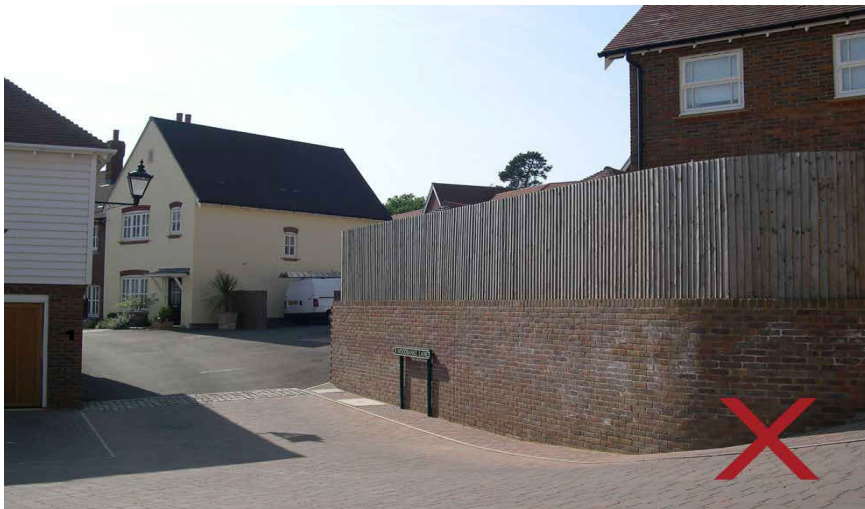
Building set back from the corner and close boarded fence with solid retaining wall prevent views of the lane.
