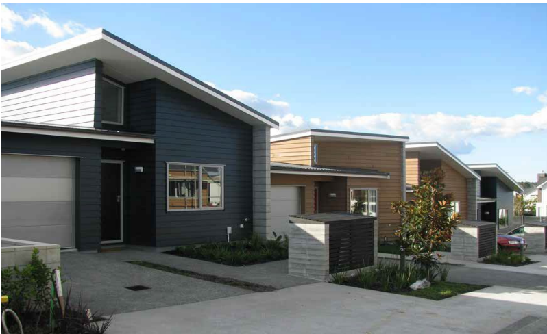
Varied roof forms create differentiation between the houses and reduce the massing of the block.
