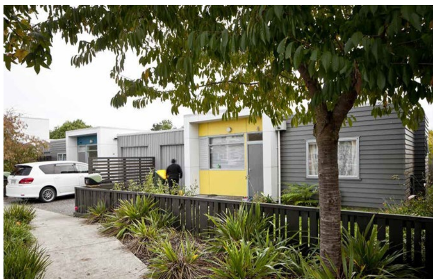
Kitchen and dining room windows provide passive surveillance over accessways and parking areas.
