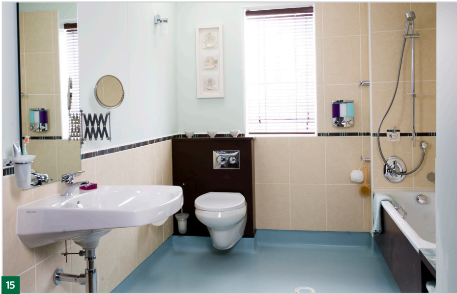
Large basin unit with work surface and space for storage of toiletries. There is space below the sink so that it can be used by a person seated.
