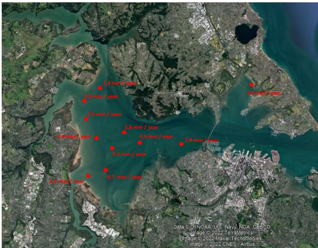
Figure 5-8 Calculated sedimentation rates (see NIWA, 2008). Locations approximate.
