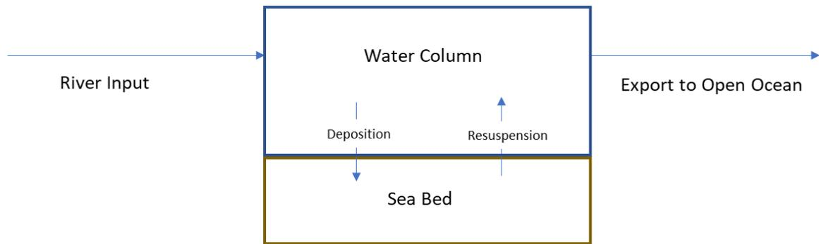
Figure 4-5 Simple overview of sediment fate model processes.
