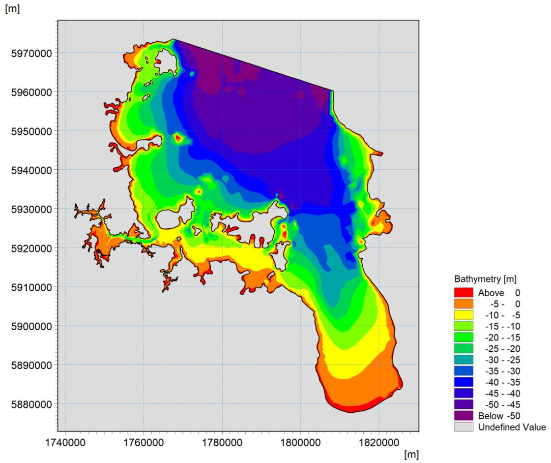
Figure 4-1 Model bathymetry and extent for inner and outer Waitematā Harbour model.
