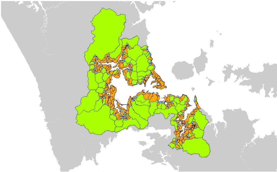
Figure 3-1 FWMT data outputs provided by Auckland Council. The green catchments link to a coastal terminal node, while orange catchments are straight to coast and have no sub-catchments upstream of them.
