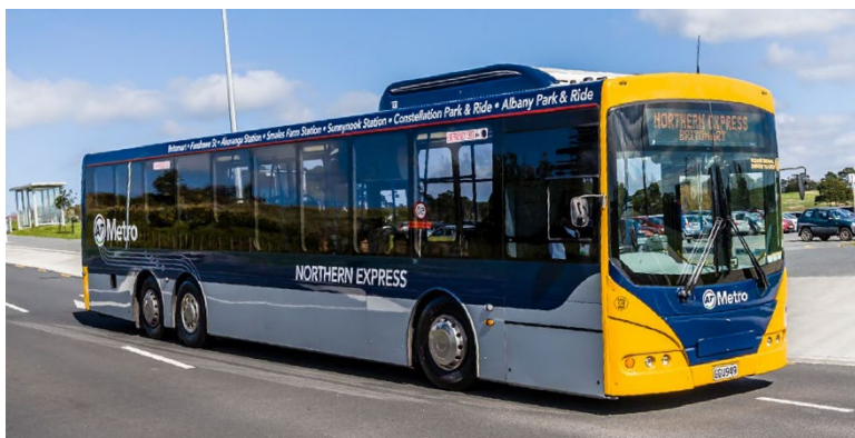
Figure 39: Typical 13.5 m AT Metro bus
