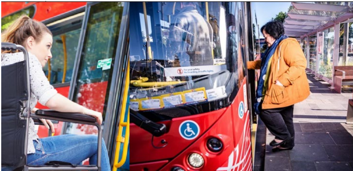
Figure 74: Small gap between the kerb and bus floor make it easy for passengers to board or alight
