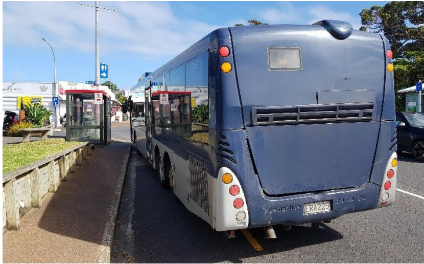
Figure 49: Failure to align bus properly and pull in at a sharp angle.
