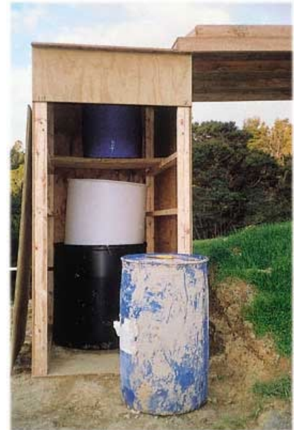
Figure 100: Rainfall activated flocculant treatment device
