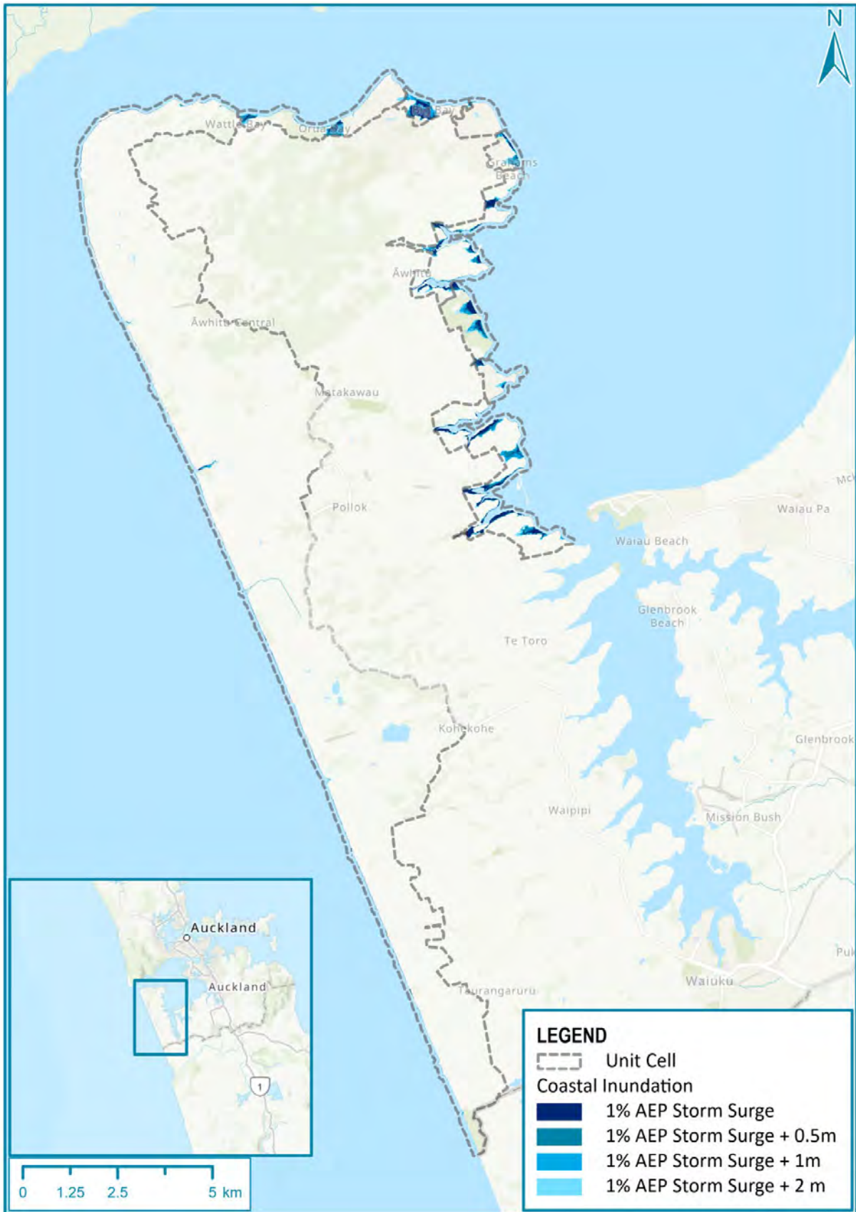
Figure 2-5: Coastal inundation for 1% AEP storm surge for present day, and with 0.5 m, 1 m, and 2 m sea-level rise
