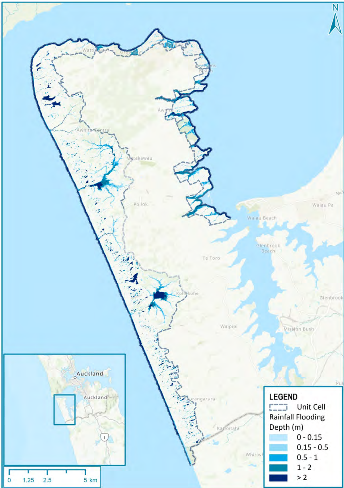
Figure 2-8: Rainfall flood extents and depths for the Maximum Probable Development, 1% AEP rainfall event with 2.10 C allowance for climate change
